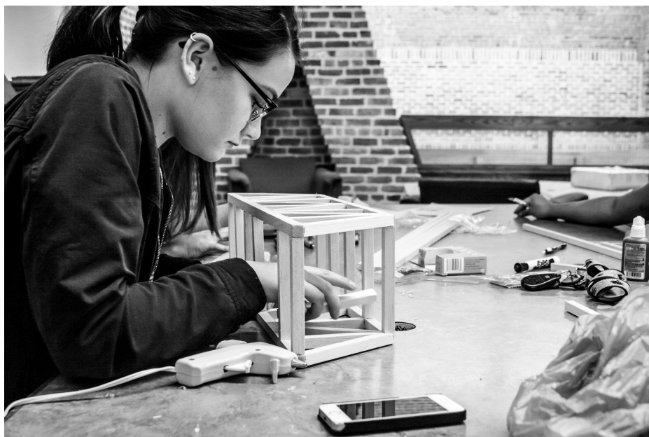
Fig. 3. A team of engineering students assembling a real-world model of a truss bridge from balsa wood structural members precision cut to their design specification; successful designs sustain can static loads far in excess of 300 pounds.
